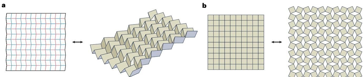
**Fig. 1 | Basic origami and kirigami patterns.** **a**, The crease pattern and the folded configuration of a standard Miura-ori pattern. The red and blue edges correspond to mountain folds and valley folds respectively. **b**, The cut pattern and the deployed configuration of a standard rotating-squares kirigami pattern.
