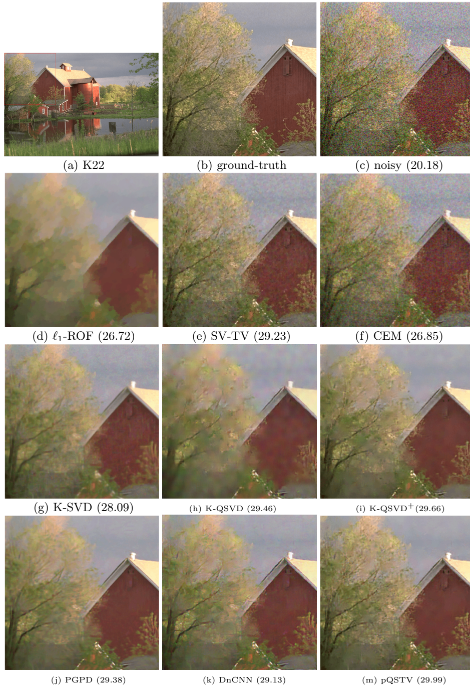
FIGURE 7. Color image denoising results on K22. (a) Original image; (b) Zooming part of the original image; (c) Noisy image corrupted by Gaussian noise with variance \sigma = 25 ; The denoised image reconstructed by: (d) \ell_1 -ROF [5], (e) SV-TV [20], (f) CEM [27], (g) K-SVD [32], (h) K-QSVD[50], (i) K-QSVD + [50], (j) PGPD [48], (k) DnCNN [56], (m) our pQSTV.
