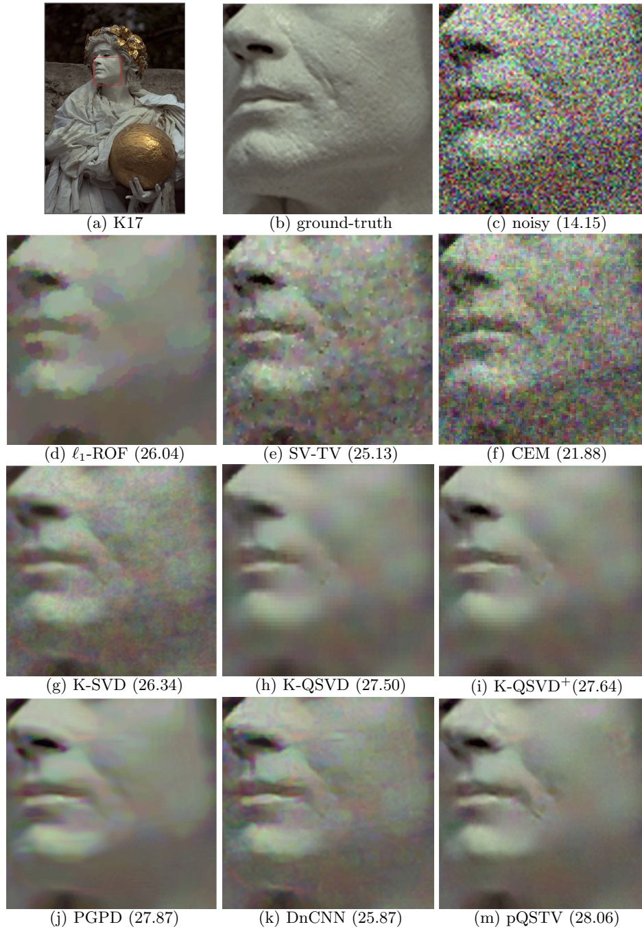
FIGURE 10. Color image denoising results on K17. (a) Original image; (b) Zooming part of the original image; (c) Noisy image corrupted by Gaussian noise with variance \sigma=50 ; The denoised image reconstructed by: (d) \ell_1 -ROF [5], (e) SV-TV [20], (f) CEM [27], (g) K-SVD [32], (h) K-QSVD[50], (i) K-QSVD + [50], (j) PGPD [48], (k) DnCNN [56], (m) our pQSTV.
