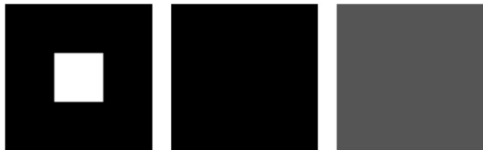
Figure 2: The images on the left and on the right are equally similar to the image in the middle in terms of the entrywise 2-norm. On the other hand, the image on the right is significant less similar to the image in the middle in terms of the entrywise 1-norm than the image on the left.
