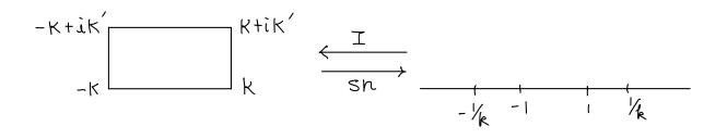
Let  $sn = I^{-1} = R \longrightarrow IH$  be the inverse conformal map. Then boundary straight line segments are map into real axis, Schwarz reflection principle extend sn(z) analytically to
