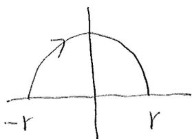
$$\text{length} = \int_{-r}^r \frac{r dx}{\sqrt{r^2 - x^2}} = 2 \int_0^r \frac{r dx}{\sqrt{r^2 - x^2}} = 2r \int_0^{\pi/2} \frac{r \cos \theta d\theta}{\sqrt{r^2 - r^2 \sin^2 \theta}}, \quad \boxed{4}$$
