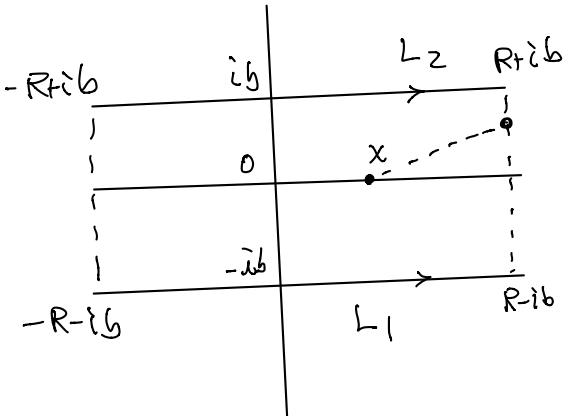
Note that  $\left| \int_{R-ib}^{R+ib} \frac{f(s)}{s-x} ds \right| \leq 2b \cdot \frac{A}{1+R^2} \cdot \frac{1}{R-x}$  for  $R > x$ .
