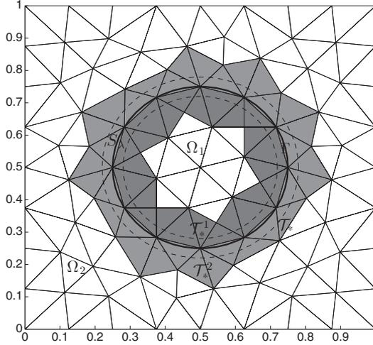
Fig. 1. An illustrative example of the finite element triangulation.
