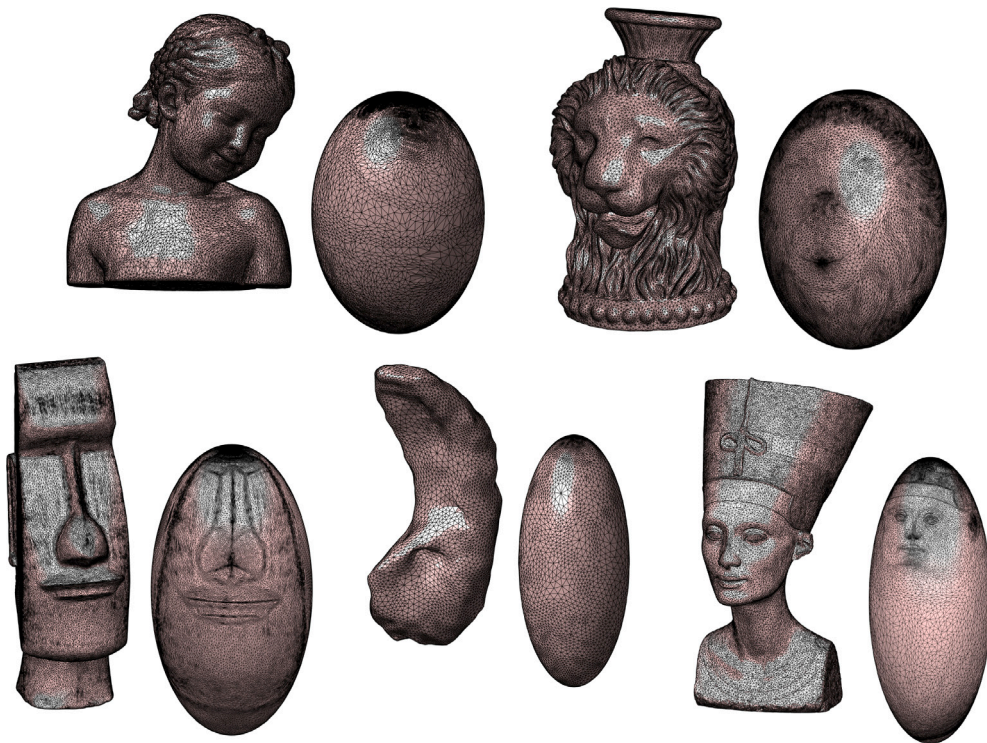
Fig. 1. Ellipsoidal conformal parameterizations obtained by our proposed framework for different genus-0 closed surfaces.
