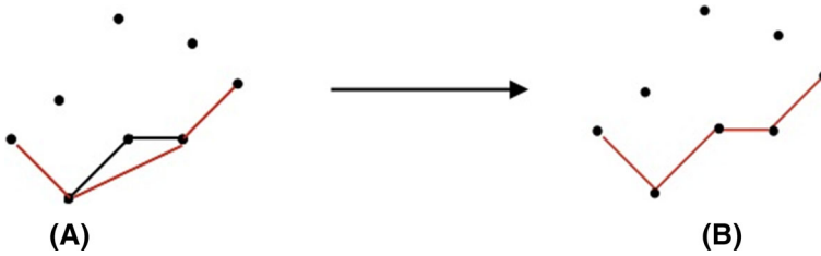
Fig. 2 Capturing the concavity of the point cloud boundary. a Boundary points captured without applying the angle criterion. b Boundary points captured with the angle criterion applied
