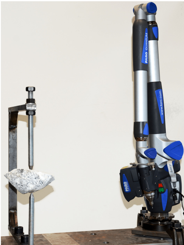
Fig. 13. The laser scanner setup using the Quantum FARO Arm®; the left side of the picture shows the laser scanner used to scan the stone, and the right side shows the stone pinned on a steel frame for the scan to minimise the loss of surface data.
