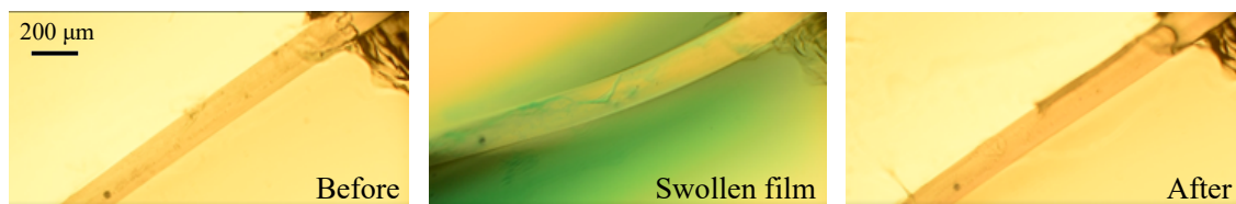
Figure S6: A PDMS film that is mounted vertically on a glass cover slip between two rigid epoxy posts swells to about 20% its original thickness when immersed in acetone (dyed with methylene blue) and reduces to its original thickness when acetone evaporates.
