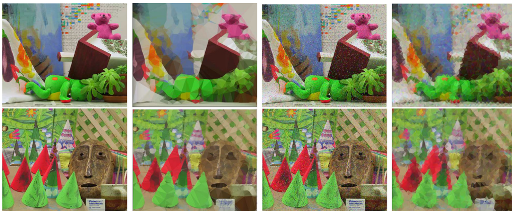
Fig. 11. Two triangulation examples by our TRIM algorithm for noisy images. Left to right: The noise-free images, the triangulations computed by TRIM based on the noise-free images, the noisy images, and The triangulations computed by TRIM based on the noisy images. Note that the important features of the images are preserved even for noisy images.
