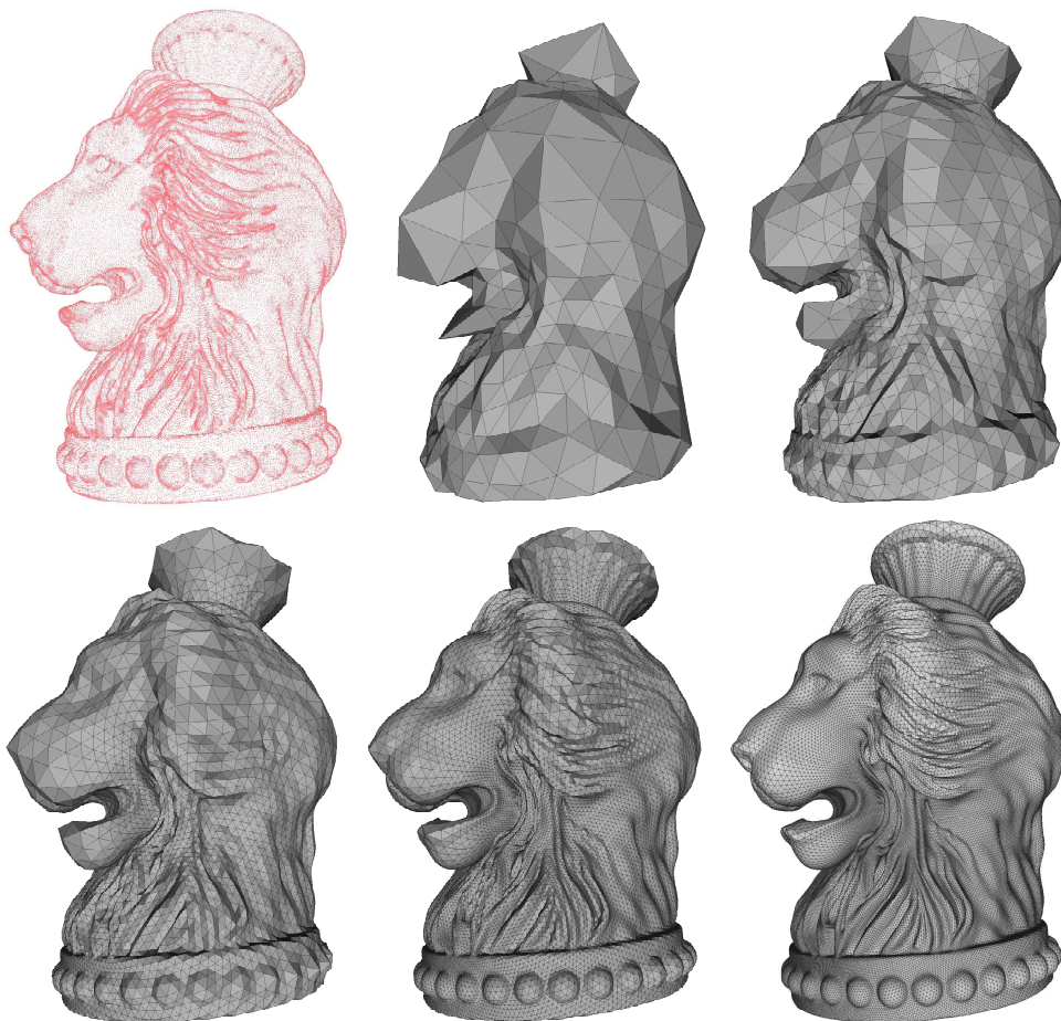
Figure 15. Multilevel representations of a genus-0 lion vase point cloud. For better visualizations, we create mesh structures on the representations. Top left: A lion vase point cloud with 256094 points. Top middle to bottom right: The multilevel representations with 0, 1, 2, 3, and 4 subdivisions. The representations are with 696, 2778, 11106, 44418, and 177666 points, respectively.
